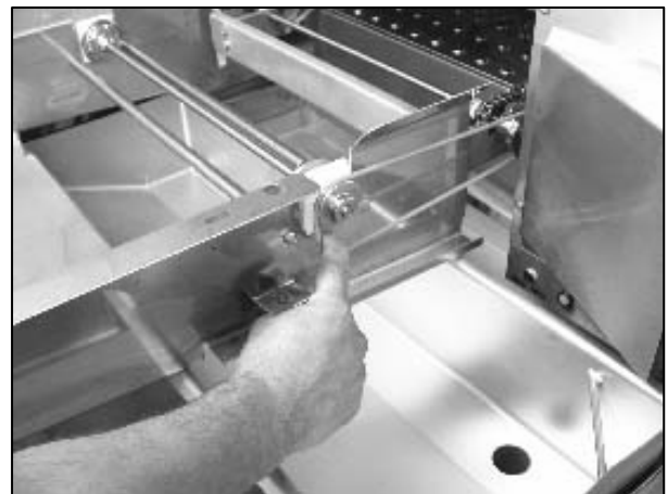
27. Connect the drive belt.
